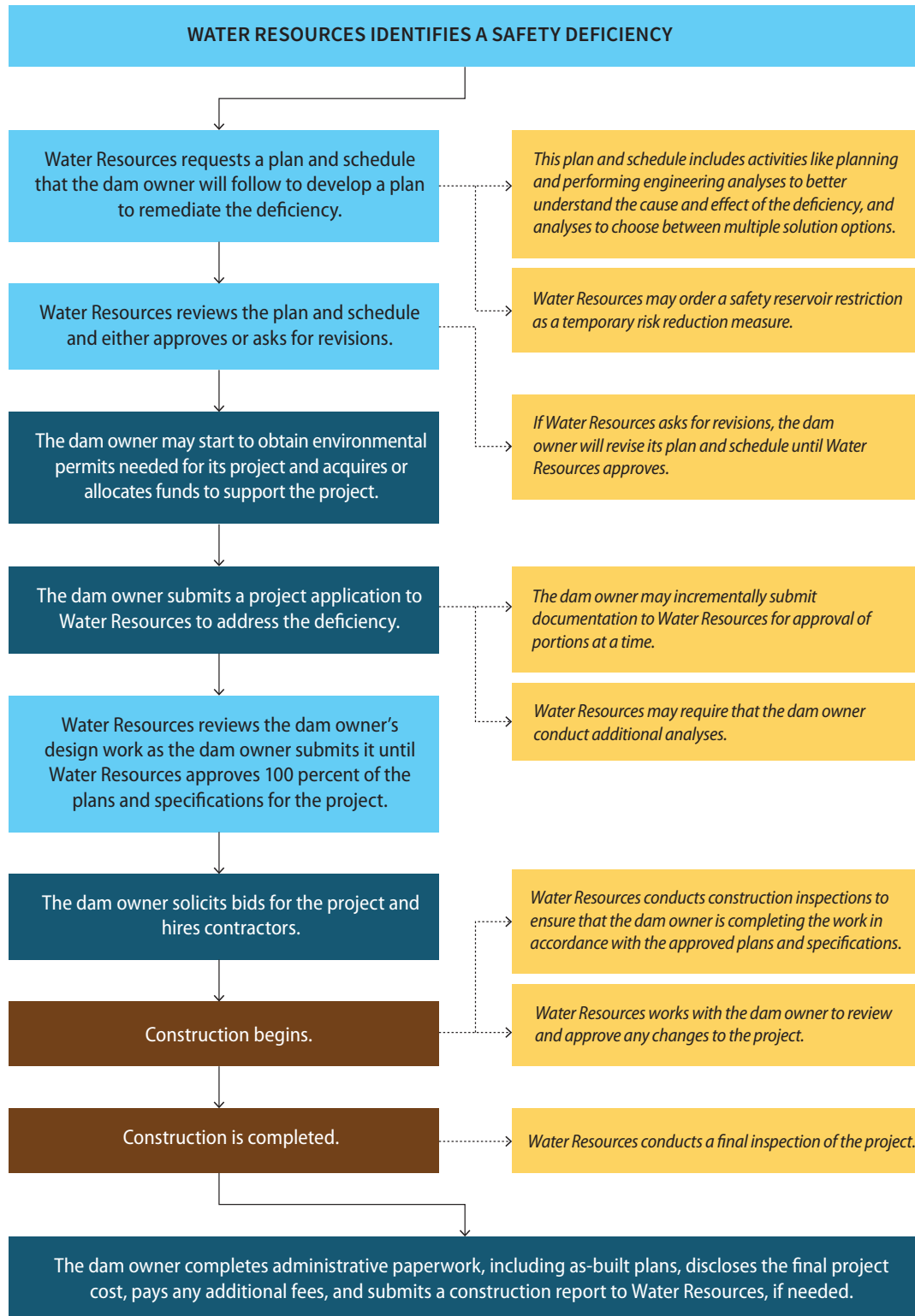
Figure 3 Dam Repair Projects Include Multiple Steps
